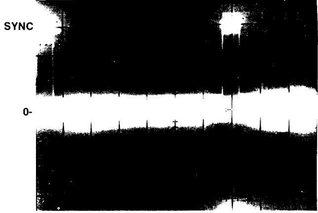
Test point: Pin 20 of ACT (U1) Time base: 0.1 ms/cm Vertical gain: 2 V/cm
